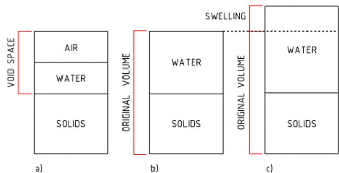
**Figure 1: a) Idealised soil structure b) Shrinkage limit: water fills the void space, total volume unchanged c) Swelling: water molecules bonded around soil particles separate the particles, increasing total volume**
