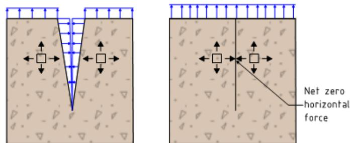
**Figure 2:** a) Soil swelling within the cracked zone, fills the cracks horizontally and causes vertical ground movement b) Cracked is closed (or below cracked zone) ground movement is only in the vertical direction.
